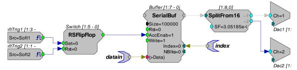
The circuit below uses a SerialBuf and SplitFrom16 to play out signals to two channels continuously. The signal is generated on the PC and then loaded into the serial buffer memory.
