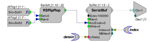
When the Soft1 trigger goes high, the FlipFlop goes high and stays high. This sets the AccEnab line high and the serial buffer starts sending the data out to the DAC. When the serial buffer has played out 100,000 points the index is reset and the data at the beginning of the buffer is played out. As long as the AccEnab is high the serial buffer will play the signal.
