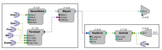
The box on the left has components that generate (GaussNoise) and filter (ParaCoef/Biquad) the waveform. The parameter tags are used to set the amplitude of the noise and filter parameters. The second part of the circuit (box on right) checks for clipping (signal values greater than  $\pm 10$  volts) and generates a high signal on Bit 0 (M=1) of the processor device if clipping occurs.
