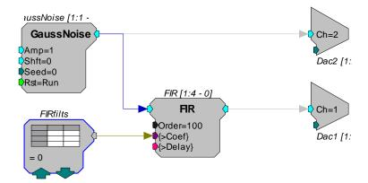
The circuit uses a GaussNoise component to output a signal. The signal is then filtered with an FIR (low, high or bandpass) filter whose coefficients are loaded from a data table. The signals are played out on Channel 1(filtered) and Channel 2(unfiltered) for comparison purposes.
