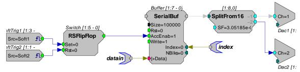
The circuit below uses a SerialBuf and SplitFrom16 to play out signals to two channels continuously. The signal is generated on the PC and then loaded into the serial buffer memory.
