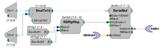
The circuit uses two AdcIns and a ShufTo16 component to acquire two channels of data continuously at 100kHz sampling rate. The signal is captured to a SerialBuffer, whose data is downloaded to the PC and stored in a file by the Visual Basic program. The first software trigger starts acquisition and the second software trigger halts acquisition.
