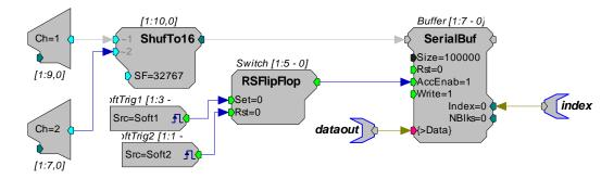
The circuit uses two AdcIns and a ShufTo16 component to acquire two channels of data continuously at 100kHz sampling rate. The signal is captured to a SerialBuffer, whose data is downloaded to the PC and stored in a file by the Visual Basic program. The first software trigger starts acquisition and the second software trigger halts acquisition.
