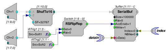
The circuit uses a SerialBuf and ShufTo16 to acquire two channels of data continuously at a 100 kHz sampling rate. The signal is captured to a serial buffer, downloaded to the PC, and stored in a file.
