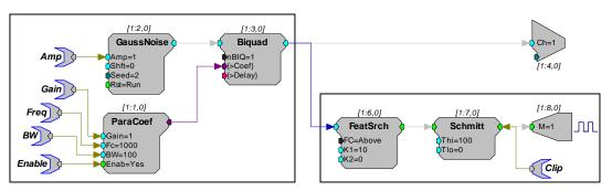
The box on the left has components that generate (GaussNoise) and filter (ParaCoef/Biquad) the waveform. The parameter tags are used to set the amplitude of the noise and filter parameters. The second part of the circuit (box on right) checks for clipping (signal values greater than +/- 10 volts) and generates a high signal on Bit 0 (M=1) of the processor device if clipping occurs.
