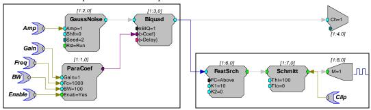
The box on the left has components that generate (GaussNoise) and filter (ParaCoef/Biquad) the waveform. The parameter tags are used to set the amplitude of the noise and filter parameters. The second part of the circuit (box on right) checks for clipping (signal values greater than  $\pm 10$  volts) and generates a high signal on Bit 0 (M=1) of the processor device.
