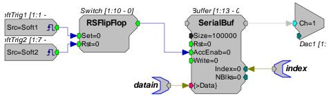
When software trigger 1 goes high the RSFlipFlop goes and stays high. This sets the AccEnab line high and the serial buffer starts sending the data out to the DAC. When the serial buffer has played out 100000 points the index is reset and the data at the beginning of the buffer is played out. As long as the AccEnab is high the Serial Buffer will play the signal.
