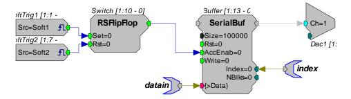
When the Soft1 trigger goes high, the FlipFlop goes high and stays high. This sets the AccEnab line high and the serial buffer starts sending the data out to the DAC. When the serial buffer has played out 100,000 points the index is reset and the data at the beginning of the buffer is played out. As long as the AccEnab is high the serial buffer will play the signal.
