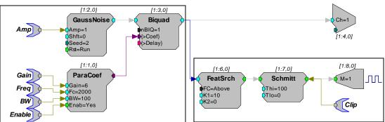
The box on the left has components that generate (GaussNoise) and filter (ParaCoef/Biquad) the waveform. The parameter tags are used to set the amplitude of the noise and filter parameters. The second part of the circuit (box on right) checks for clipping (signal values greater than  $\pm$ 10 volts) and generates a high signal on Bit 0 (M=1) of the processor device.
