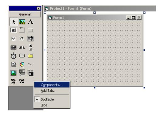
4. In the dialog box, click the **Controls** tab. Scroll down the list and select the **RPcoX ActiveX Control module** check box, then click **OK**.
